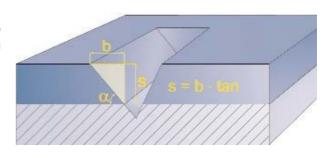
For adhesion tests in accordance with AS 1580 Meth. 408.1, the width of the area where the coating has flaked off during the cutting operation is related to projection b.
